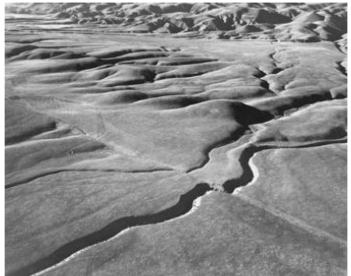
Fig. 4.1-1 Aerial photograph of the San Andreas fault in the Carrizo Plain in California, seen from the south. Note the displacement of stream gullies as the Pacific plate ( near side ) has moved to the left (northwest) relative to North America. (Copyright John S. Shelton.)
