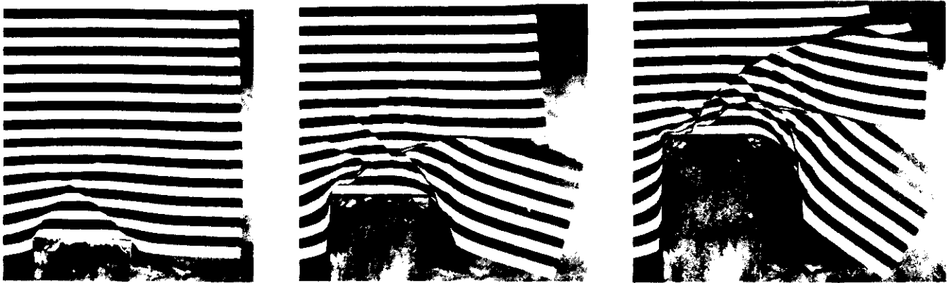
Fig. 5.6-7 Demonstration of the deformation of Asia, modeled by a striped block of plasticine, as the result of a collision with a rigid block simulating the Indian subcontinent. The plasticine is constrained on the left side, so the impact forces blocks to be extruded to the right, analogous to the eastward motion of blocks in Indochina and China. (Tapponnier et al. , 1982. Geology , 10, 611–16, with permission of the publisher, the Geological Society of America, Boulder, Co. © 1982 Geological Society of America.)
